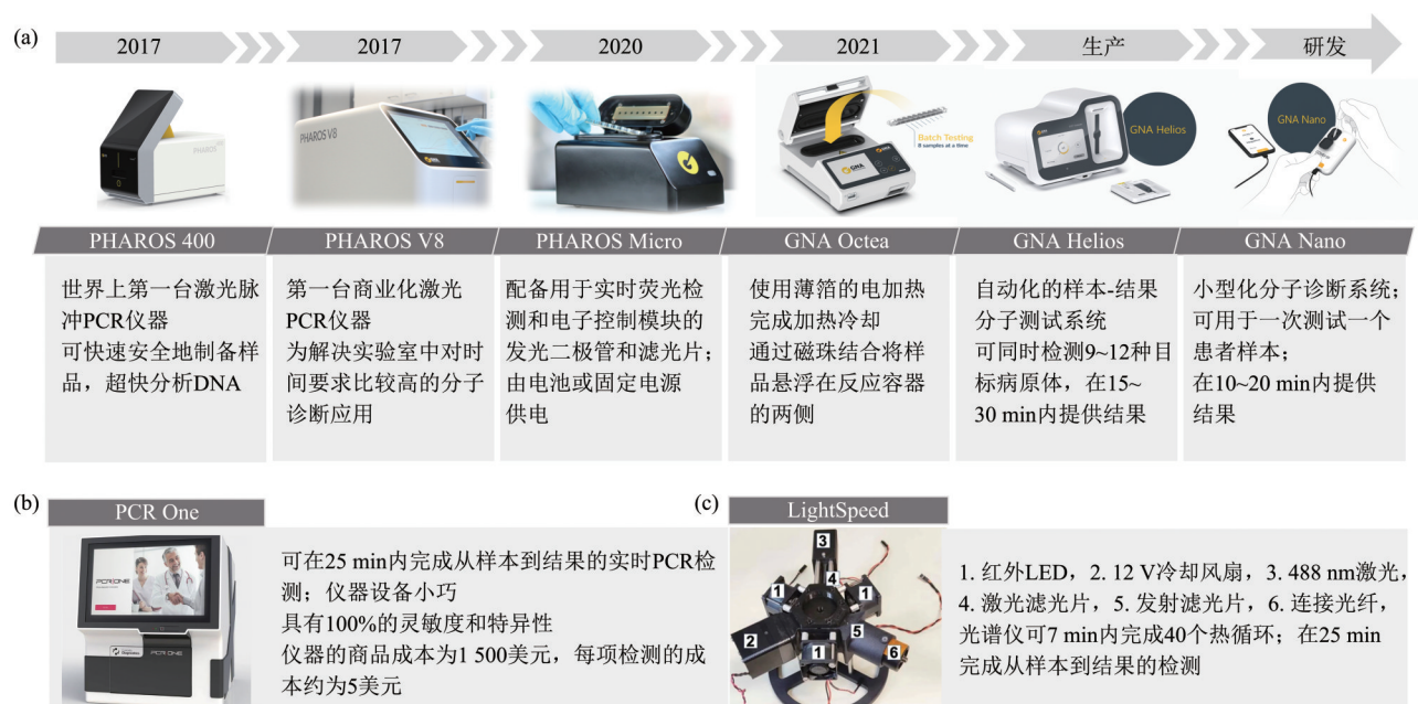
Fig. 4 Development of equipment for ultra-fast pulse-controlled PCR technology
